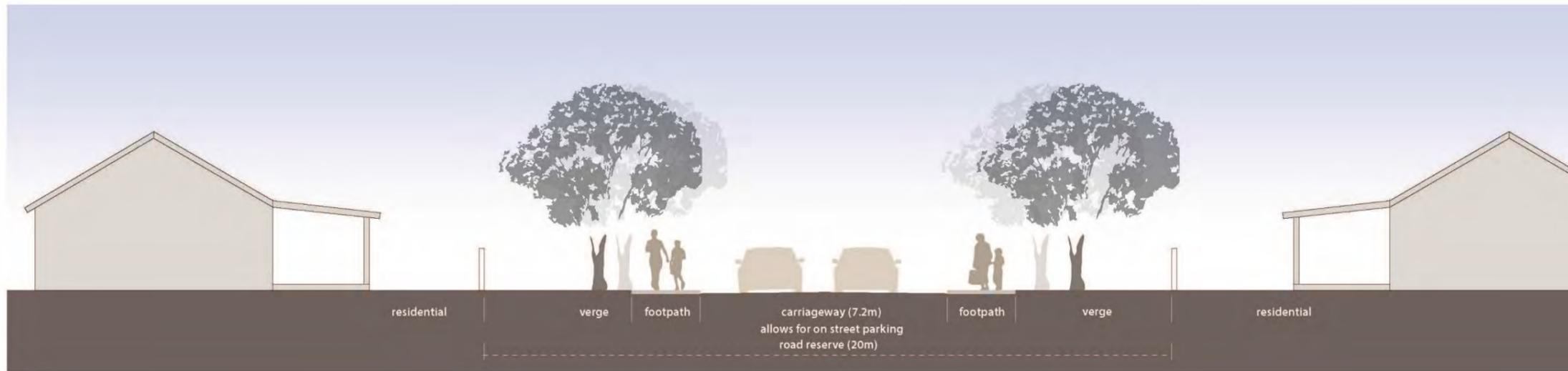
Figure 7 – Indicative cross section for typical local roads
