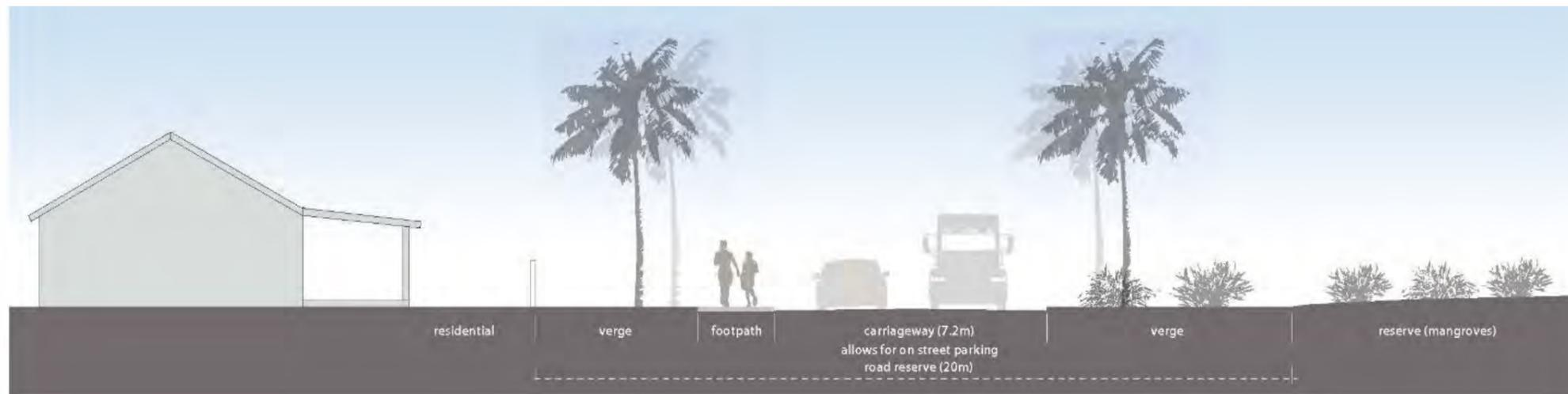
Figure 8 – Indicative cross section for main entry roads
