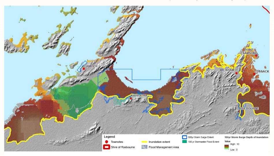
Figure 32: Stormwater flood extent and storm surge extent modelling (Strategen, 2013)
