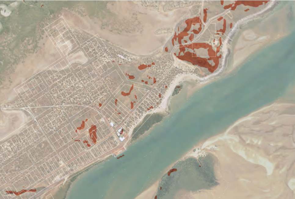
Slope analysis: Areas steeper than 1:10 (10%) are in red.
