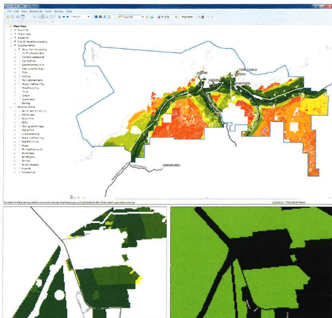
Figure 3-3 Screenshot of data interrogation tool for evaluating site suitability surfaces, with focus on Gap Ridge / Karratha Airport region.
