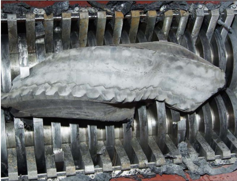
Image 1:2 Typical Shredder Blades
