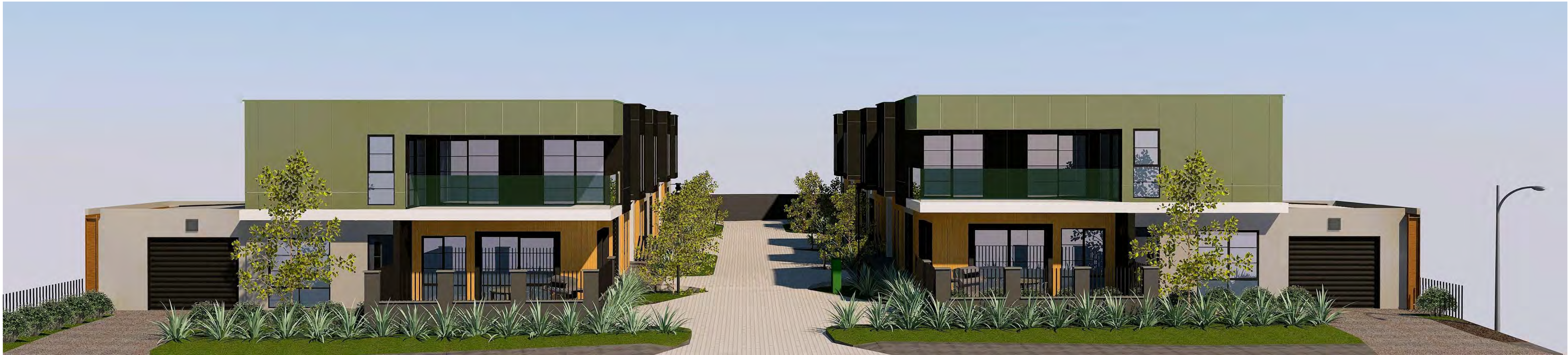
1 NORTH ELEVATION #LayID / Scale 1:100 1. RAINWATER SPILLWAY 2. 2400 HIGH ROLLER DOOR 3. SENSOR LIGHTING 4. LEVEL ENTRY - 1200 x 1200mm MIN 5. SENSOR LIGHTING OVER ENTRY 6. VISUAL CONNECTION TO STREET 7. SECURE COURTYARD 8. BALCONY OVERLOOKING STREET 9. INTERNAL LAMP POST 10. BOUNDARY SCREENING 1200mm HIGH 11. MAIL BOX 12. INTERNAL DRIVEWAY 13. CAR PORT 14. STORE 15. ROOF FALL TO REAR 16. PARTITION WALL (HEBEL INFILL FIRE RATED) 17. WALL ON BOUNDARY (FIRE RATED) 18. SECURE COURTYARD WALL 1800mm HIGH 19. OPAQUE GLAZING 20. GLAZING 1600mm AFL 21. BOLLARD LAMP (TIMER) 22. NEATA SCREEN FENCING 1800mm HIGH
