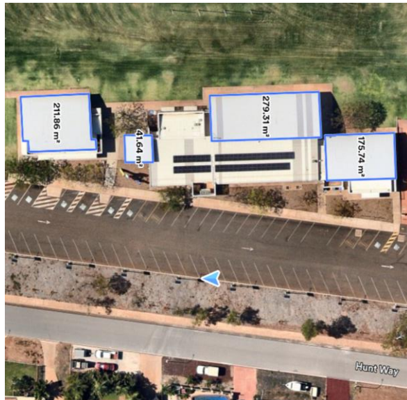
FIGURE 27: AERIAL VIEW AND AVAILABLE ROOFTOP AREA FOR FRANK BUTLER RESERVE AND COMMUNITY CENTRE
