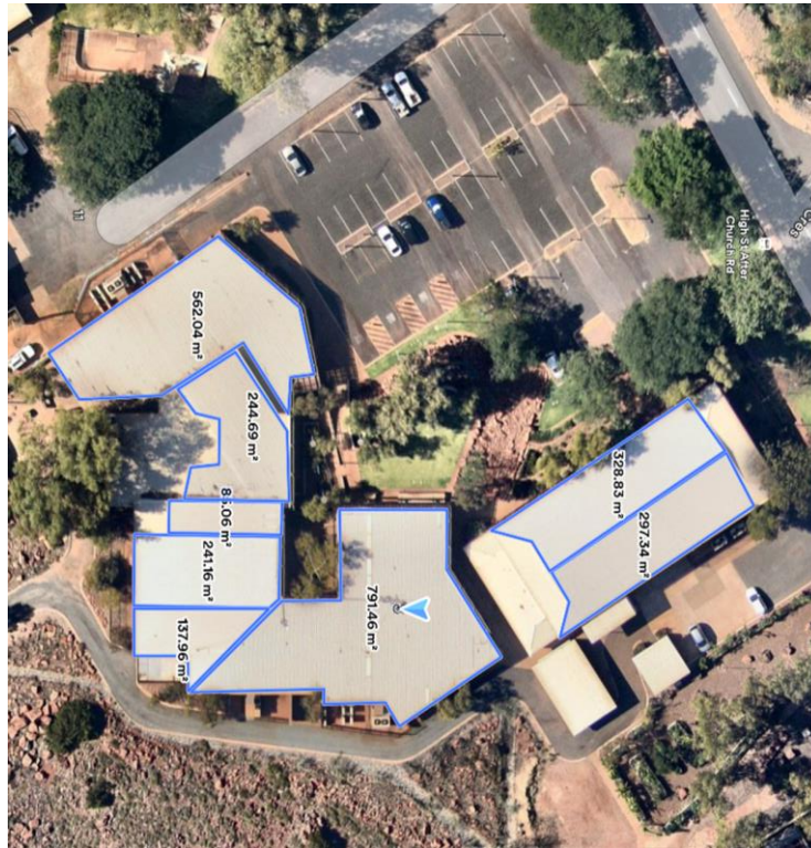
FIGURE 23: AERIAL VIEW AND AVAILABLE ROOFTOP AREA OF DAMPIER COMMUNITY CENTRE
