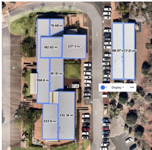
FIGURE 21: AERIAL VIEW AND AVAILABLE ROOFTOP AREA OF ADMIN BUILDING
